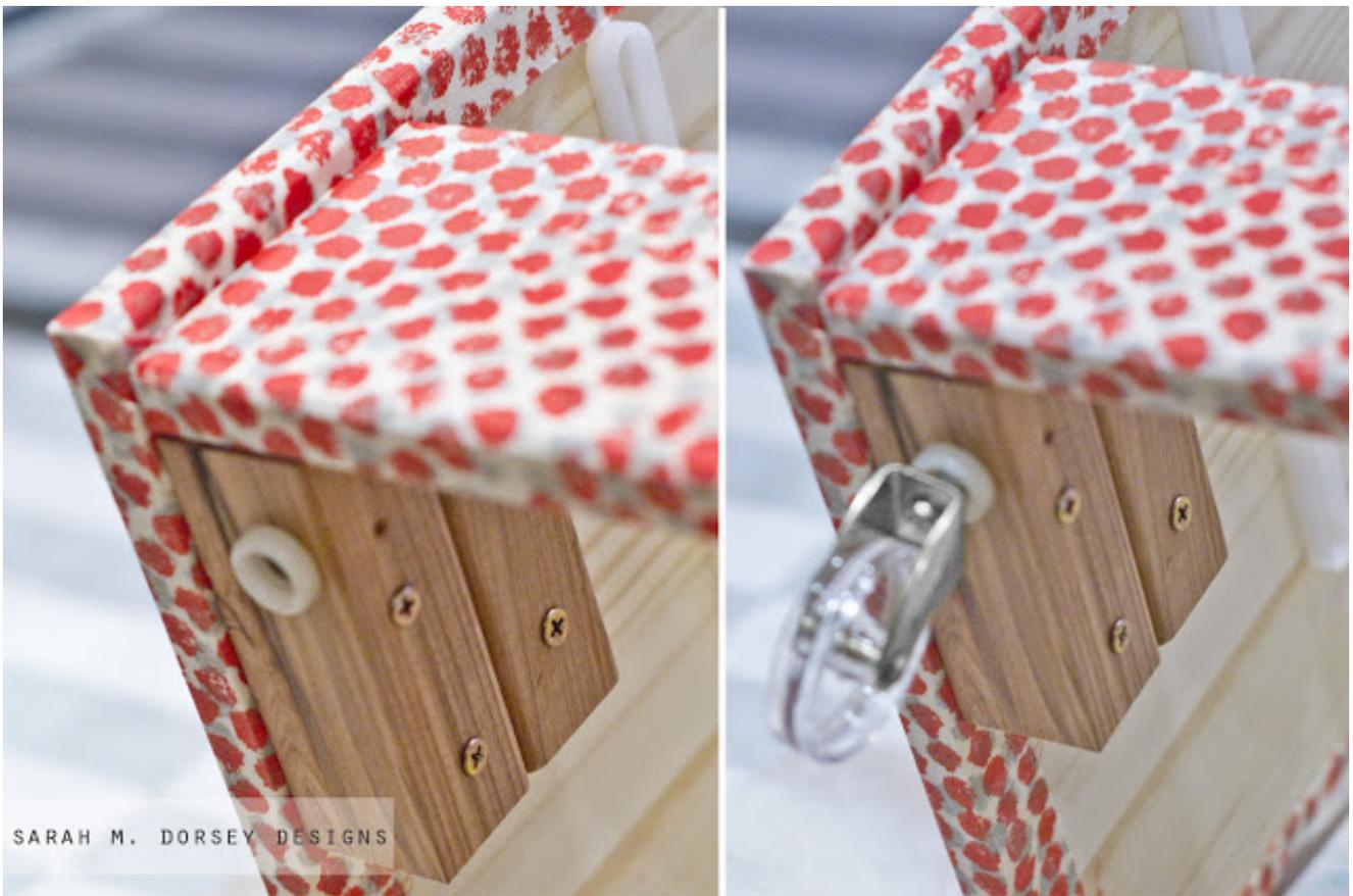
Before assembling the dresser, David drilled new holes to make the plate below the drawers flush instead of inset. We installed supports for casters out of extra 2x2s and followed the instructions to install the casters. We found brass and clear plastic casters from Ace Hardware, love them!! I then applied silver rub n buff to match the ring pulls.
