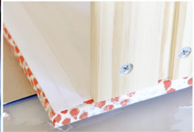
We ended up wrapping the pieces individually, which meant the sides the top needed to be attached first with the fabric between the top and side since the screw holes are exposed and then insert the screws, and then apply poly and iron. It would be quicker to assemble the entire outside and then wrap that verse the individual pieces, so also consider doing it that way. I don't think that it would of looked very different, but would save time :)
