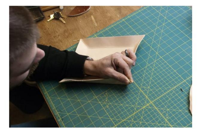
4. Next, fold the leather on the embossed the line. This is to encourage the leather to hold the desired shape when the corners are pinched together.
