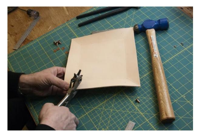
7. Next, make some holes in each corner for the rivets. Paul uses a revolving hole punch, which you can buy at a good hardware store. Or, if you are feeling courageous, cut the holes carefully with the tip of an X-Acto knife.
