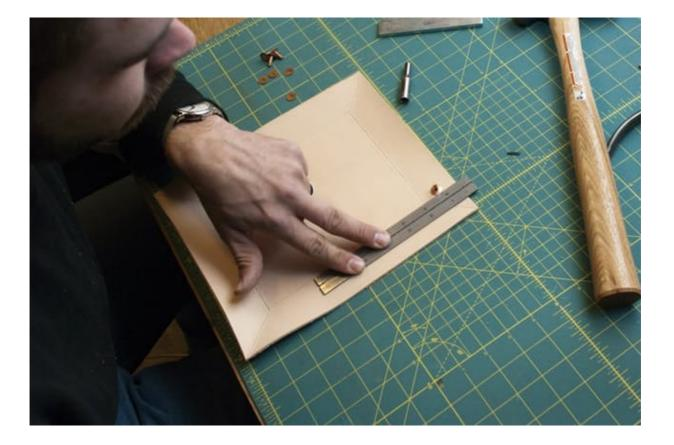
Figure out where to place the rivets. Just remember, the rivets will actually pinch and hold the leather together about an 1/8 inch beyond the edge of the rivet head. If you've never worked with rivets before, buy a few extra and practice on a scrap piece of leather before you do this step.
